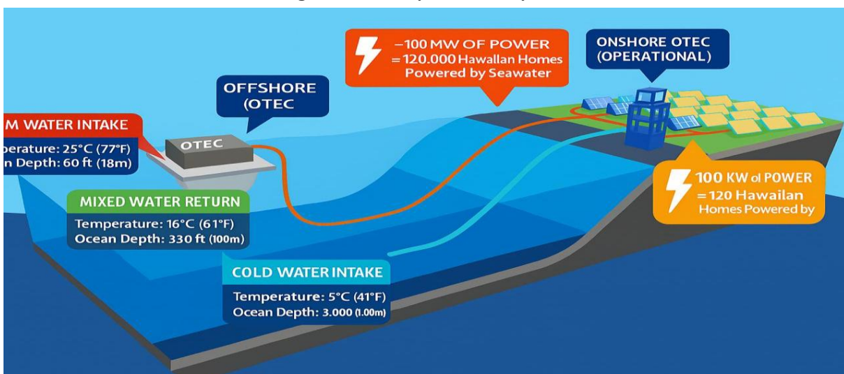
Fig. 2.2 Ocean Thermal Energy Conversion (OTEC) system
